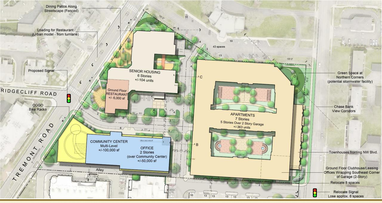
Ground Level Plan / Site Plan
