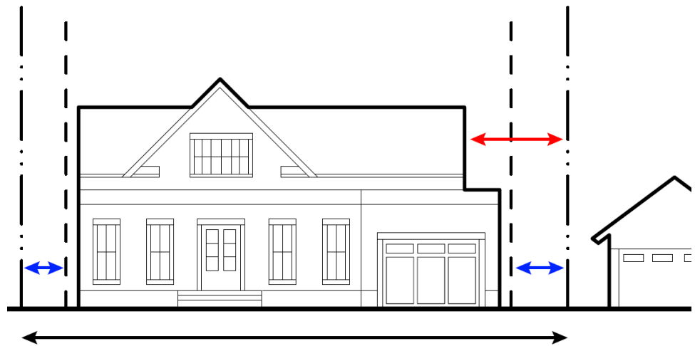
Figure 6: A new home has the second story stepped-back when adjacent to a single-story home.
