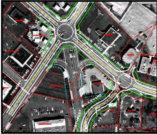
Realigned Northwest Boulevard with Two Roundabouts on Fishingner Road
