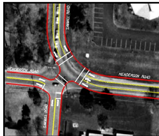
Realigned Sawmill and Henderson Roads
