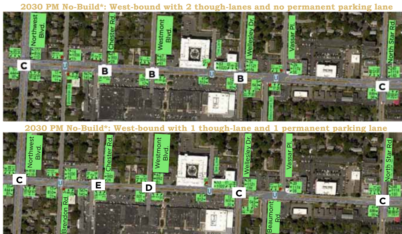
FIGURE 2: Level of Service Comparison Diagram * No-build: this study ignores future development within the PMUD and applies only anticipated peripheral growth.
